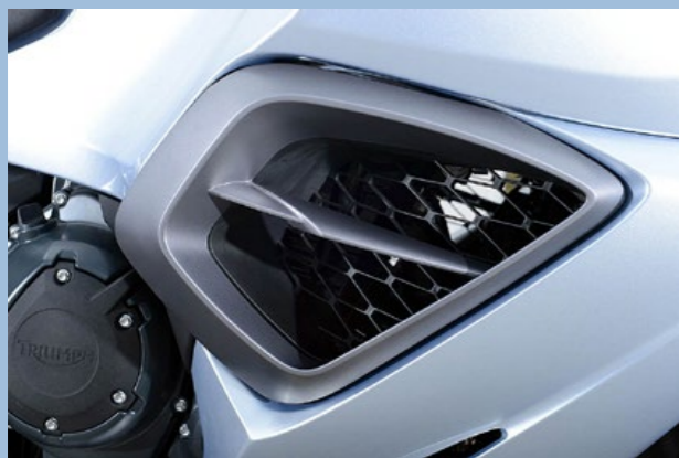
Hot air from engine is routed away from rider's legs via side air duct.
