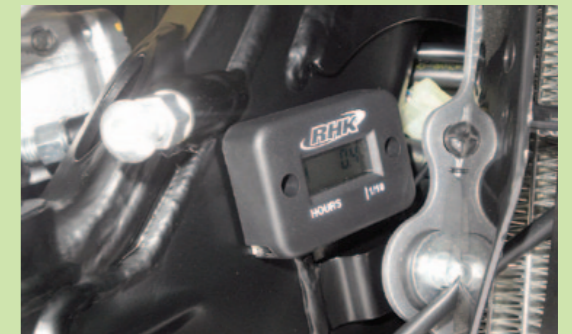
An hour meter is a better indicator of when oil changes are needed than the odometer.
