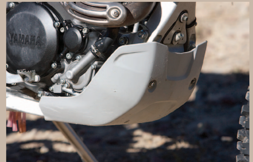
Plastic bash plate offers some protection, but not enough for hard riders.
