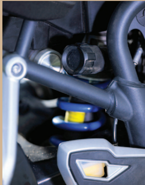
Rear shock pre-load changes are via the handy hydraulic adjuster.
