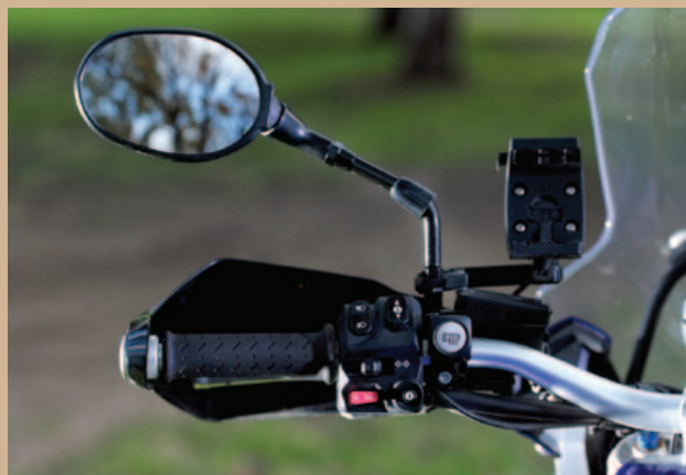
Left switchblock house loads of buttons so you can heat your hands and turn the traction control off for example.
