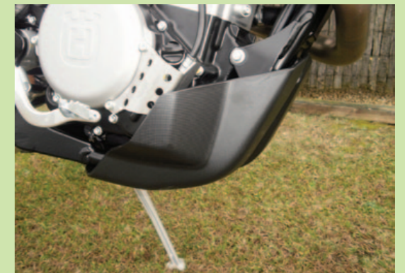
While the original plastic bash plate is sturdy I think an alloy unit will replace it.
