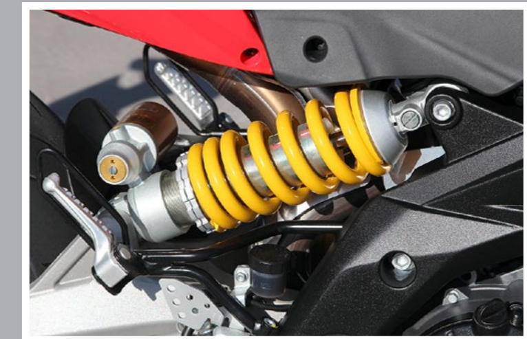
Sidemounted Sachs shock is fully adjustable.
