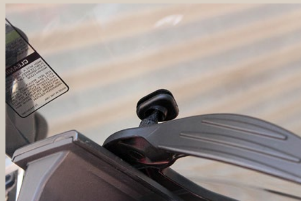
The quick-release screen mounting system.
