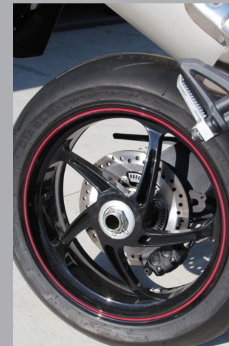
Forged alloy wheels are lighter than the standard model.
