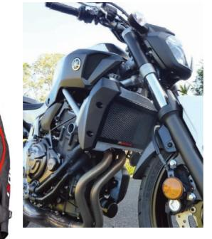
Guards are made out of high grade aluminium; the expanded mesh is used to protect the radiator core along with a rigid frame that also acts as a brace. The Rad Guards are bolted onto an existing mount point on one side of the bike and held in place on the other side by the Yamaha's pin system. Available in Polished Alloy or Powder Coated Black. Check out their website to view the fitting instructions video.
