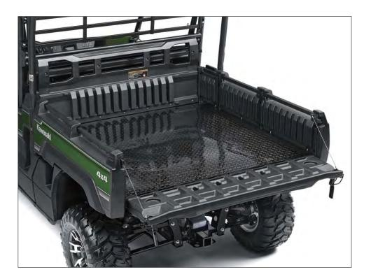
\* Gas-assisted tilting cargo bed facilitates accessing the engine. (Photo 1)
