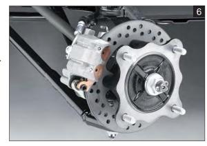
\* The rear discs, also ø212 mm, are slowed by single-piston calipers with ø34 mm pistons. (Photo 7)
