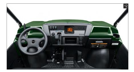
\* Clean dashboard design includes switches for the lamps, selectable 4WD, and rear differential lock. Five additional spaces for optional additional accessory switches have been prepared. (Photos 12-13)
